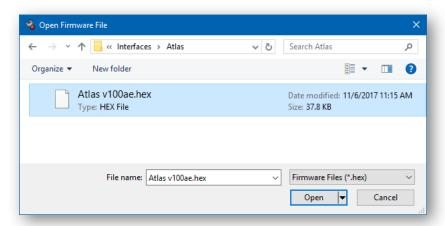
Simply select the appropriate firmware file you wish to upload to the unit and click on Open. The Atlas Firmware Uploader will now show the firmware file in the Firmware File box as shown at left:
