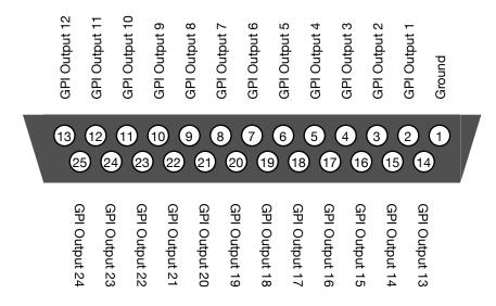
**Pinout For CMOS GPI Inputs**
