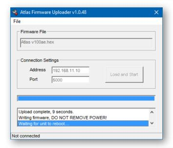
When the Atlas Firmware Uploader has completed transferring the firmware data, the utility will disconnect from the unit.
