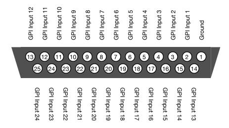
**Pinout For CMOS GPI Inputs**
