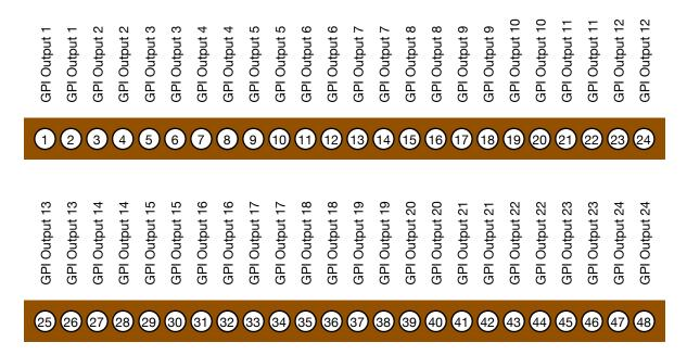
**Pinout For Optoisolator GPI Inputs**
