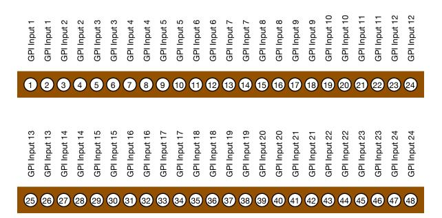
**Pinout For Optoisolator GPI Inputs**
