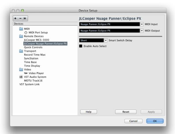
To test the operation of the panner in Nuendo, open a Nuendo project then open the Mixer Console. Locate and select surround track and make sure the mini-surround panner is visible. Press the button on the JLCooper panner's joystick then move the joystick and you should see the sound source move in the mini-panner.
