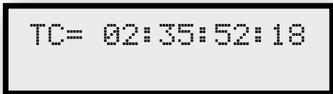
Drop Frame Timecode display in Instant Replay and Cue and Park Modes
