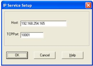
17. Enter the IP address and TCP port of your Ethernet controller. This is the Local Port you entered in the XPort Installer or Device Installer. If you configured a different port number in the XPort Installer or Device Installer application, enter that number in the TCPPort box. Click OK.
