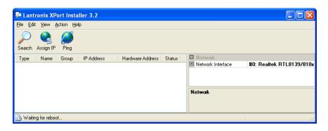
6. Your device will disappear momentarily from the XPort Installer window and reappear. During this time, the status bar in the bottom left corner of the window will display "Waiting for reboot...".
