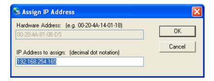
5. Enter the IP address you want assigned to your Ethernet Controller and click OK. In this example, we are using 192.168.254.165 however, you can use any address.
