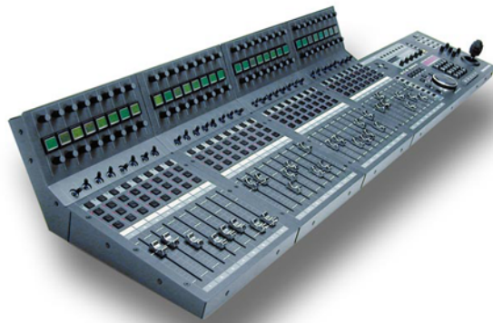
MCS-3800 with three MCS-300 fader expanders, four MCS-Bridges and an MCS-Panner
