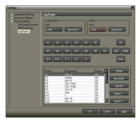
In the Fader section, set the COM port that appeared in the Device Manager.
