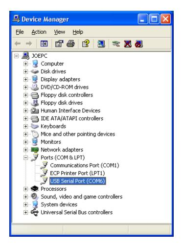
2. Look for the item "USB Serial Port". There will be a COM port next to it. This is the COM port associated with your FaderMaster 4/100. You will use this to specify which COM port your application will use to access the FaderMaster 4/100. Close the Device Manager.
