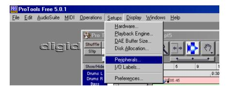
Select the MIDI Controllers tab and set Type to HUI. You will need to specify the MIDI port where your FaderMaster 4/100 is plugged into. The FaderMaster 4/100 will now control your on screen faders. Additionally, the faders on the FaderMaster 4/100 will move just like the on screen faders in response to automation.
